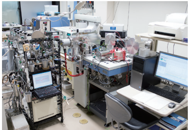
Isotope Ratio Mass Spectrometer
