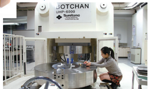
The world's largest multi-anvil apparatus and polycrystalline diamond installed at the Ehime University satellite.
